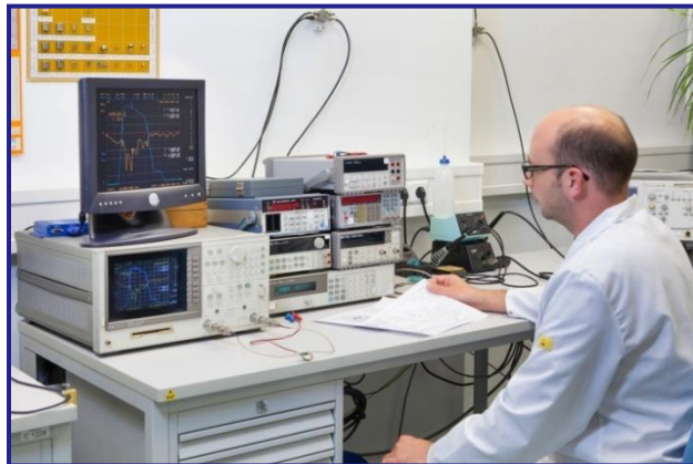
Electrical test systems for oscillators & SAW
