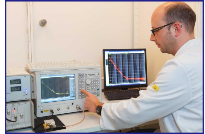
Phase noise test systems in shielded chamber
